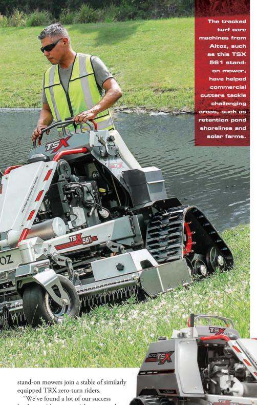
has been with commercial cutters and municipalities. With our high speed tracked vehicles - both the sitdown and the stand-on - they've found that they can mow areas they couldn't traditionally mow with a wheeled mower because
