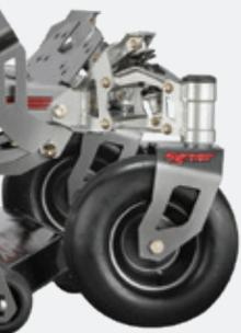
XE SS and XR SS models feature a double arm adjustable coil spring over gas shock front suspension. Available as an accessory on other XE and XR models.
