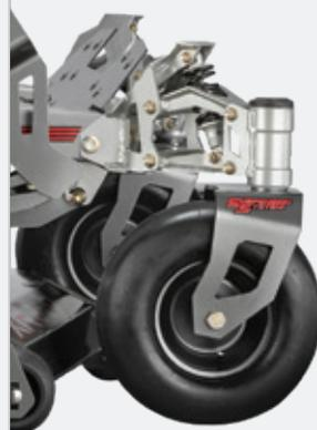
The Altoz Independent Front Suspension (IFS) smooths out rough terrain for superb comfort and control. Available as an accessory on TRX 354 models.
