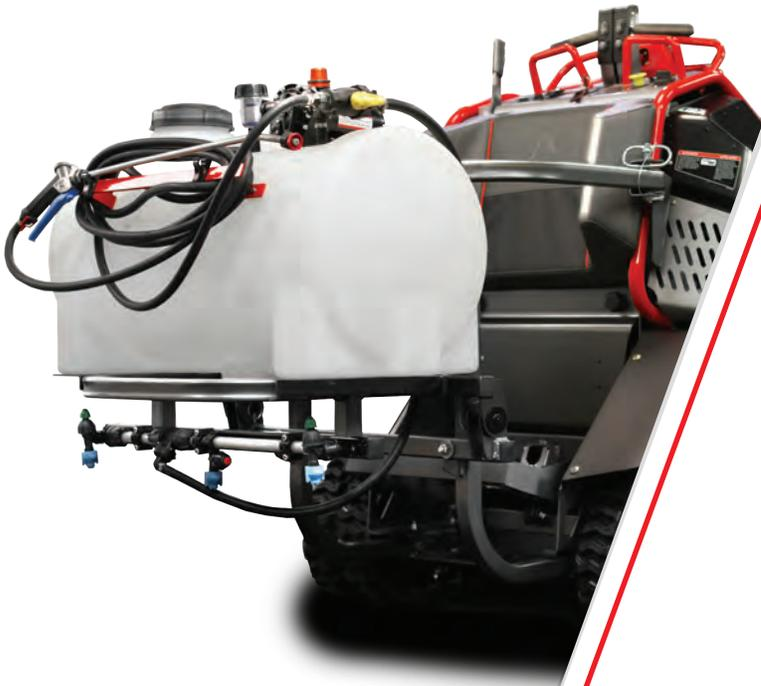
*Shown with 4' Wide Spray Pattern Brine Boom with Hypro nozzles & Rear Attachment Mount Kit*
