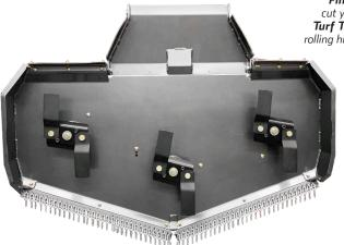
TSX models are available with the industry-exclusive 7-gauge laminated, manufactured deck featuring multi-bearing cast steel spindles and pivoting swing blades.
