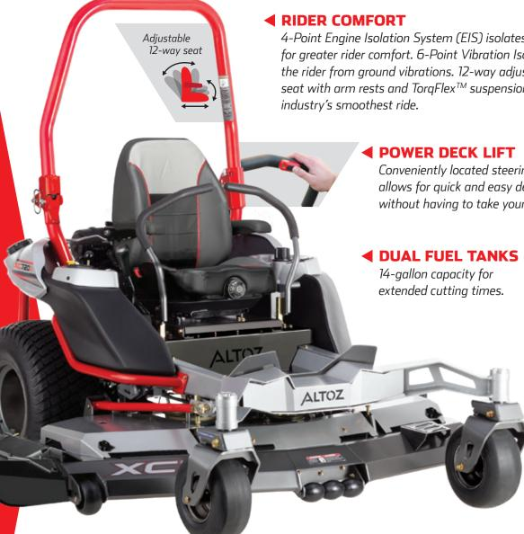
4-Point Engine Isolation System (EIS) isolates and absorbs engine vibrations for greater rider comfort. 6-Point Vibration Isolation System (VIS) isolates the rider from ground vibrations. 12-way adjustable high-back suspension seat with arm rests and TorqFlex<sup>TM</sup> suspension work together to deliver the
