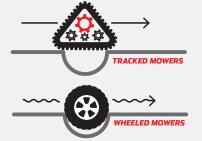
The patented TRX rear torsion axle track system delivers maximum traction for stability and low ground pressure for minimal compaction. 10" wide TerraFlex tracks are ideal for customers who cut in demanding conditions. The 11" wide All-Terrain tracks are ideal for side hilling, soft terrain and rough areas other mowers can't reach. Optional Turf Tracks are less aggressive and perfect for soft ground, rolling hills and sensitive terrain.
