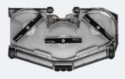
The exclusive Aero Deck is .270" fabricated steel and features fully adjustable baffles, enabling you to customize your cut to various grass conditions.
