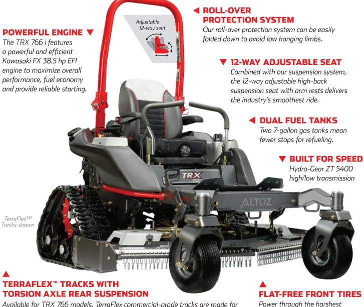
Available for TRX 766 models, TerraFlex commercial-grade tracks are made for customers who cut in demanding conditions. The tread pattern and steel-cased, vulcanized rubber tracks are designed for durability and flexibility. These tracks, combined with the torsion axle rear suspension, are engineered for traction, stability and a smooth ride in challenaing conditions.
