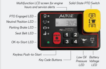
The SmarTrac<sup>™</sup> Pro control features a solid-state PTO switch, patented SoftStart clutch control that decreases mechanical wear and significantly increases deck belt life, a keyless push-to-start ignition, a large multifunction LCD screen and 6 ultra-bright status LEDs.
