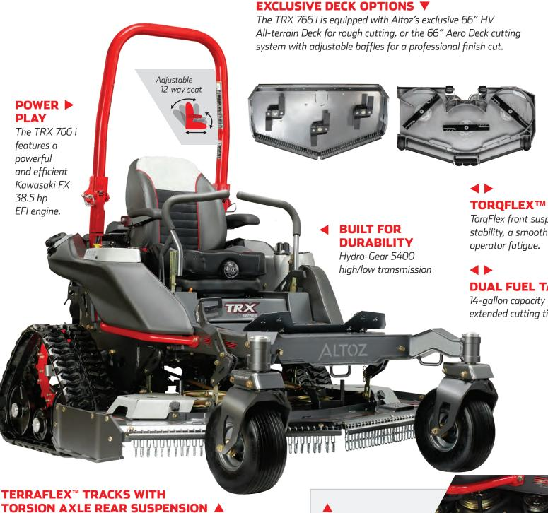
Available for TRX 766 models, TerraFlex commercial-grade tracks are made for customers who cut in demanding conditions. The tread pattern and steel-cased, vulcanized rubber tracks are designed for durability and flexibility. These tracks, combined with the torsion axle rear suspension, are engineered for traction, stability and a smooth ride in challenging conditions.
