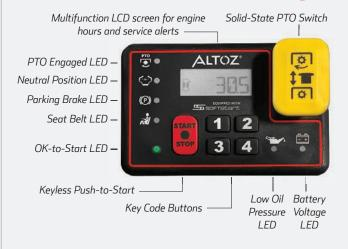
The SmarTrac<sup>™</sup> Pro control features a solid-state PTO switch, patented SoftStart clutch control that decreases mechanical wear and significantly increases deck belt life, a keyless push-to-start ignition, a large multifunction LCD screen and 6 ultra-bright status LEDs.
