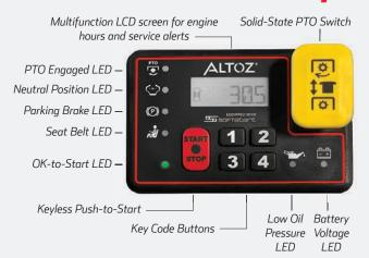
The SmarTrac™ Pro control features a solid-state PTO switch, patented SoftStart clutch control that decreases mechanical wear and significantly increases deck belt life, a keyless push-to-start ignition, a large multifunction LCD screen and 6 ultra-bright status LEDs.
