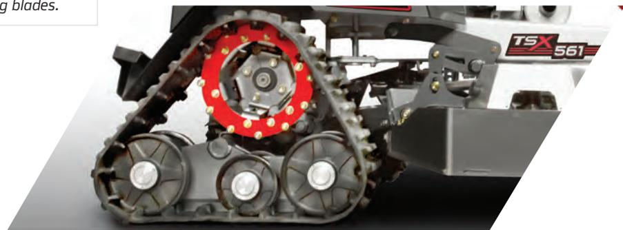
Power through the harshest conditions and rough terrain with flat-free tires and rear-mounted torsional axle suspension and track system.
