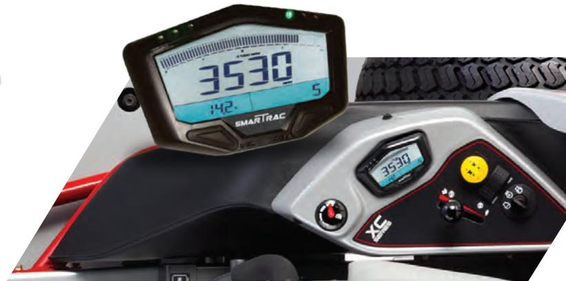
SmarTrac™ Monitoring System features a tachometer and resettable hour meter, with alerts for low oil pressure and overheating.
