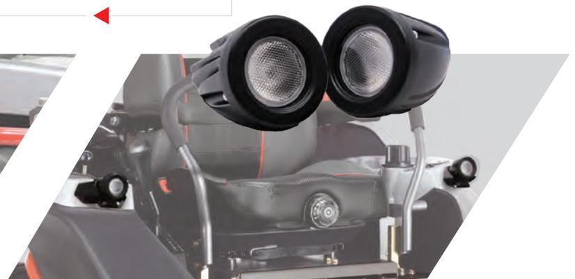
Lighting kit includes 2 LED lights built in an aluminum, shock-proof, waterproof casing. Each light provides 950 lumens with a spot beam of 25 degrees.
