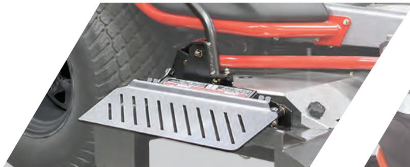
Operator-controlled discharge cover allows you to open and close the outlet quickly while mowing.
