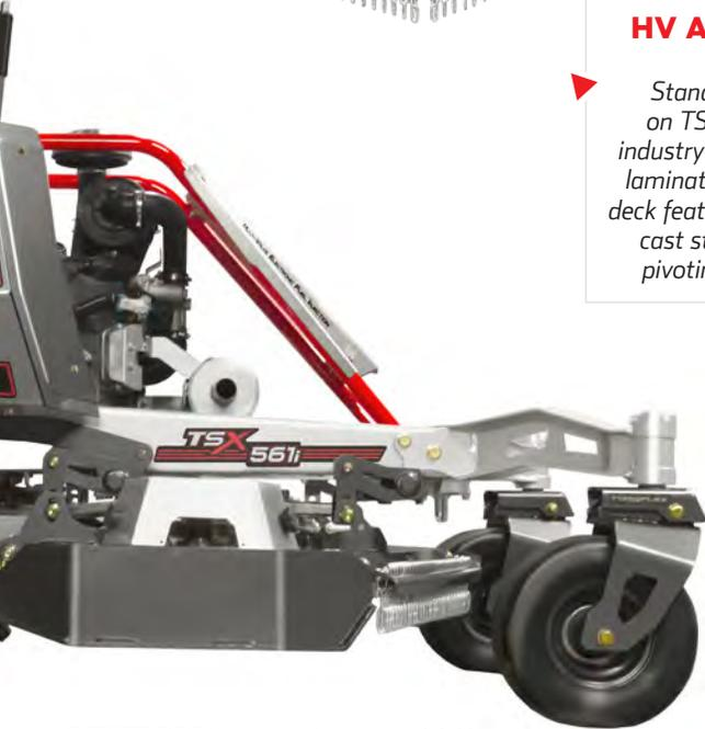
**OFFSET DECK** – Allows for better visibility on the trim side for a closer cut underneath and around immobile objects. Equipped with an industry exclusive six pivoting swing blades -- forged and heat-treated for exceptional long-lasting sharpness.
