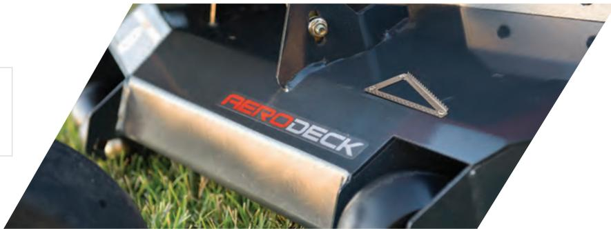
Our exclusive fabricated steel Aero Deck™ features anti-scalp wheels and fully adjustable baffles to customize your cut for various grass conditions. Available in 54" and 61" widths.
