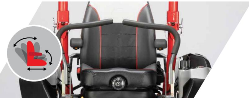
Combined with our suspension system, the 12-way adjustable high-back suspension seat with arm rests delivers the industry's smoothest ride.
